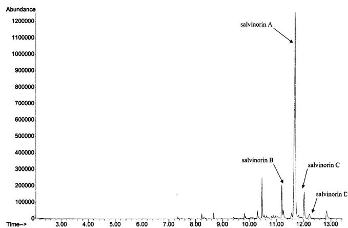
FIG. 2—Reconstructed total ion chromatogram of *Salvia divinorum* extracted by ambient temperature chloroform.
