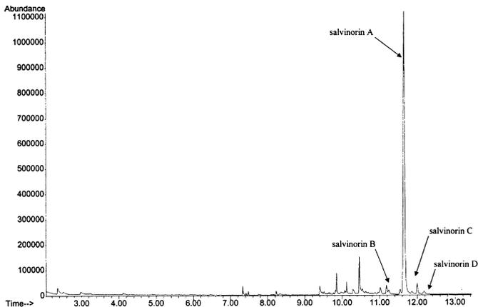
FIG. 3—Reconstructed total ion chromatogram of *Salvia divinorum* extracted by ambient temperature acetone.
